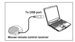
The remote control may fail to operate if the mouse remote control receiver is exposed to bright sunlight or fluorescent lighting.
